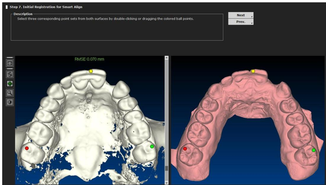
Fig. 350 Dots are placed in a triangular shape with RMSE of 0.070 mm
