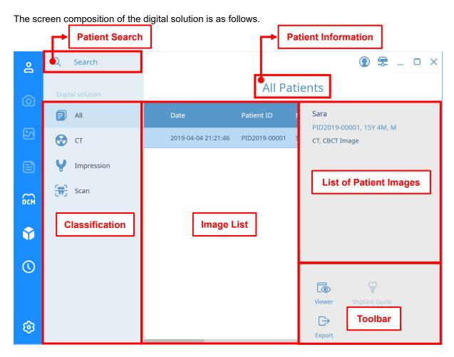
Fig 42 'Digital Solution' Tab Screen
