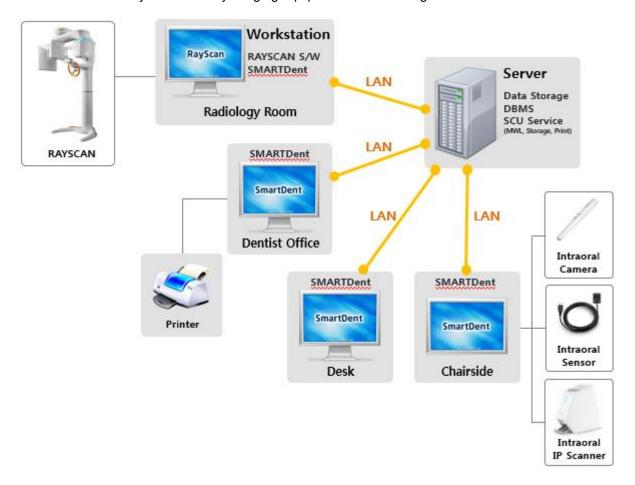
Fig 1 SMARTDent Software System Configuration
